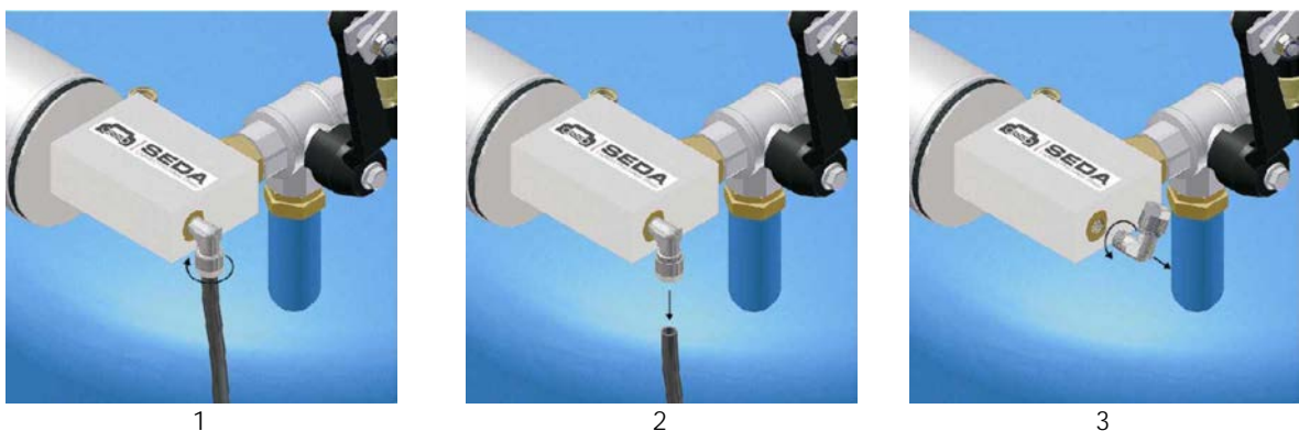
Abb. 1, 2 und 3: First loosen the air pressure hose and then remove the small angle pipe.
